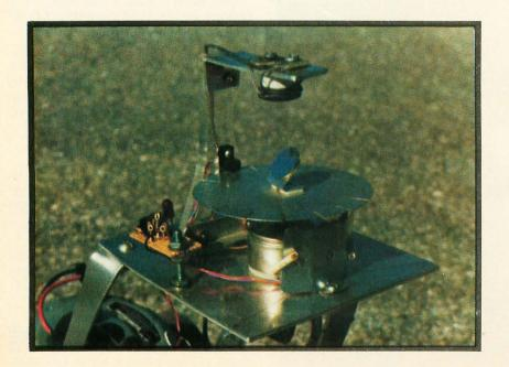
Photo 1: The primary sensor of Tee Toddler is this photoelectric horizon scanner. The "eye" mounted on a Plexiglas standard and metal bracket scans a 360° field. The flat mirror rotates at five revolutions per second deflecting light into the phototransistor eye through a 45° angle. The position of the mirror is resolved into one of 16 angular states by a slotted disk which passes through an optocoupler.
