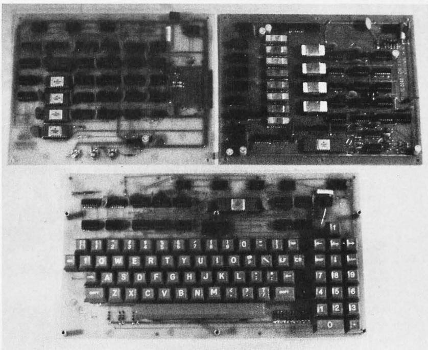
*Photo 2: Here are the three main boards of the Sphere system. At the upper left is the video interface board with 512 bytes of memory used for the display. At upper right is the main processor board with the 6800, 4 KB of dynamic memory and 1 KB of EROM. The lower board is the keyboard assembly, which includes a numerical keypad and cursor control keys as well as a full alphanumeric keyboard.*
