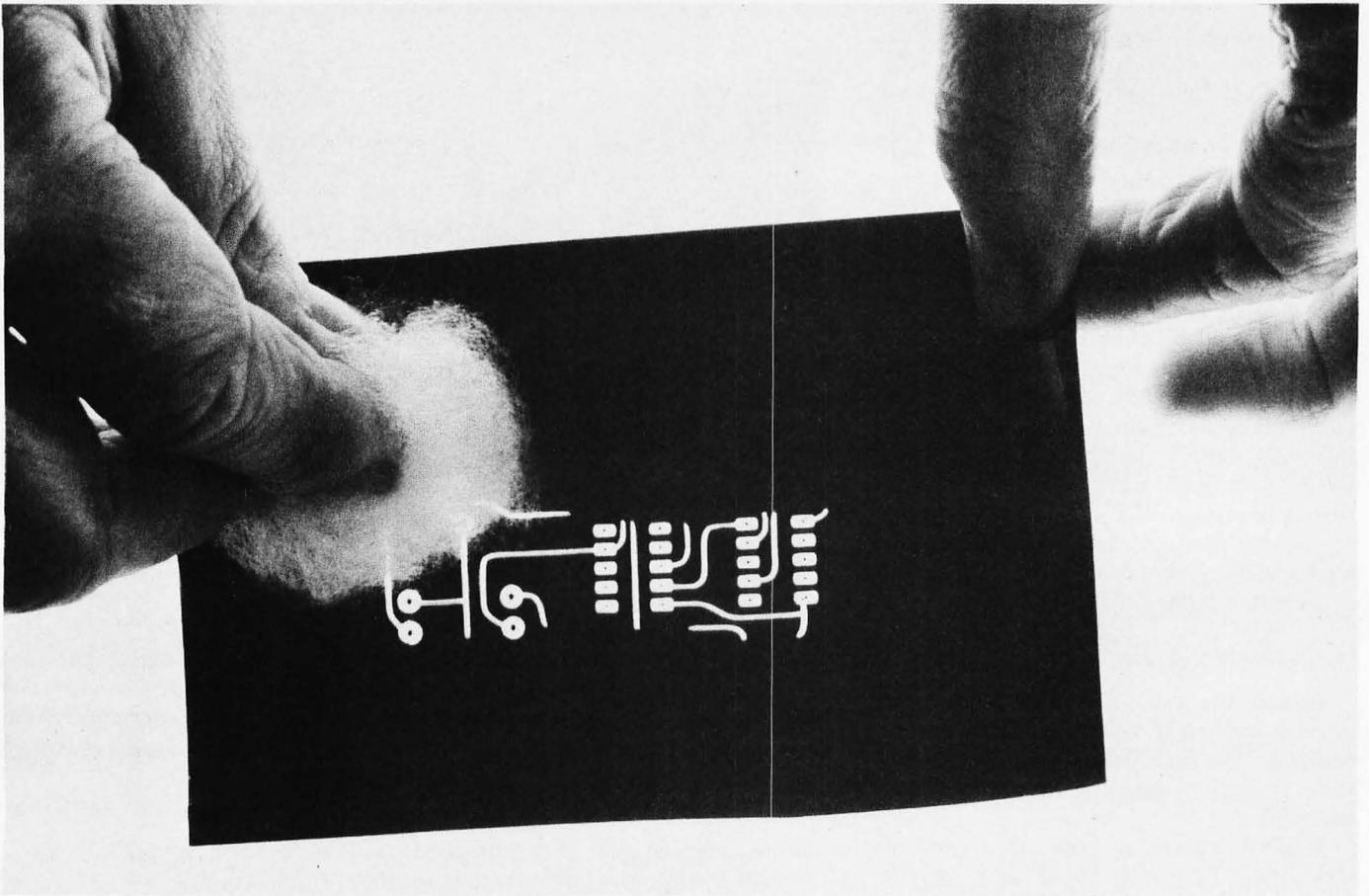
*Photo 7: Creating a Photo Negative for Etching. A negative is reproduced from the positive artwork pattern, using a reversing film. The film is exposed with a bright light, then developed by rubbing gently with a cotton swab and developing solution. The result is a negative version of the artwork with a 1:1 scaling.*
