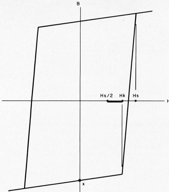
Figure 8: The half-select current  $i/2$  must generate an  $H$  field less than  $H_k$  if a change of state is to be avoided. Similarly, the full select current of  $i$  must generate an  $H$  field strength greater than  $H_s$  to ensure switching. This leaves a range of field strengths (and corresponding current values) from  $H_s/2$  to  $H_k$  which introduces a critical tolerance for the select currents in a core memory design.
