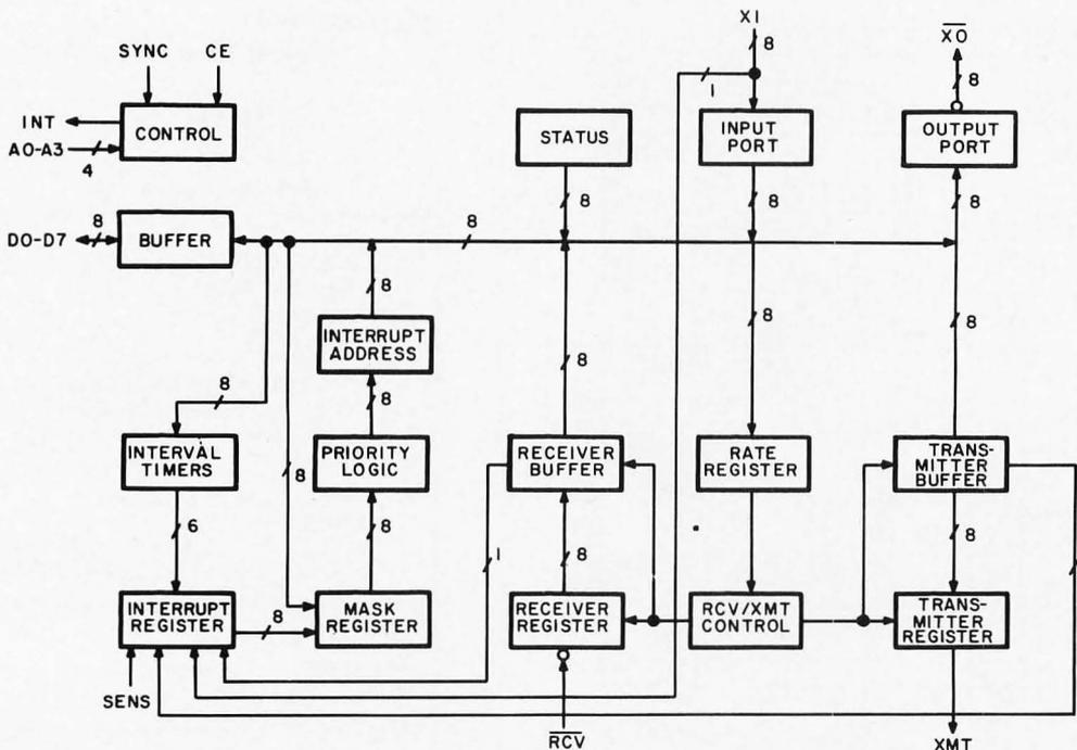
Figure 1: Block Diagram of the Texas Instruments TMS-5501 Design. This diagram shows the elements which are contained within this "do everything" IO chip. Notations next to the interconnection lines specify the number of bits involved in the data path.
