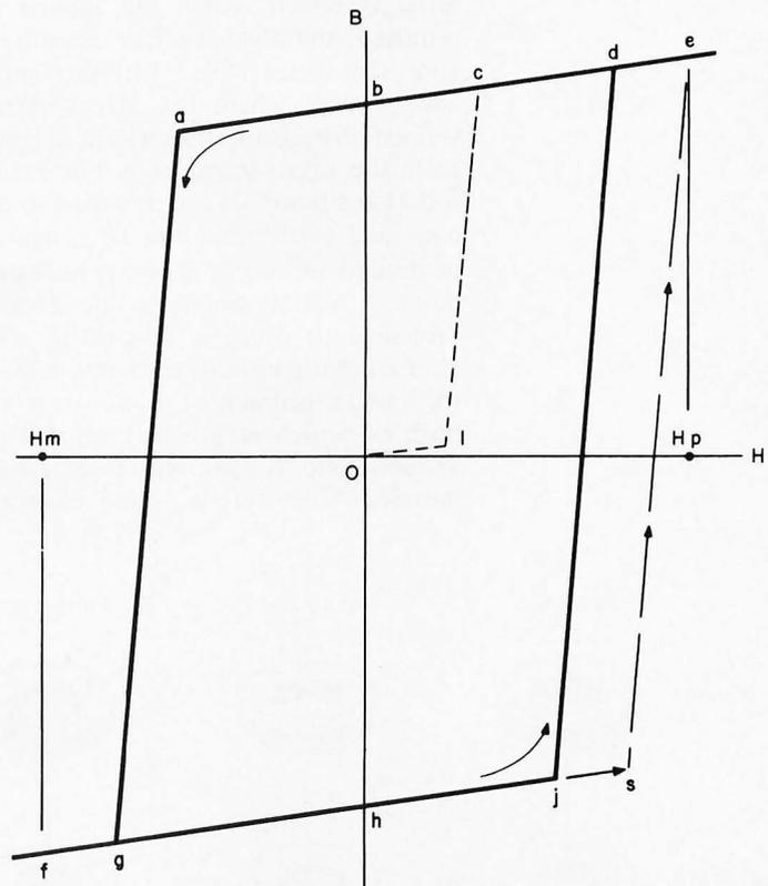
Figure 3: Memory properties are derived from the hysteresis properties of the core material. When the applied  $\mathbf{H}$  value is 0, the residual  $\mathbf{B}$  value in the core material will depend upon the past history of magnetization. This figure and subsequent figures show the magnitude of the vector quantities  $\mathbf{H}$  and  $\mathbf{B}$ , with positive and negative values corresponding to the two directions of rotation about the core axis.
