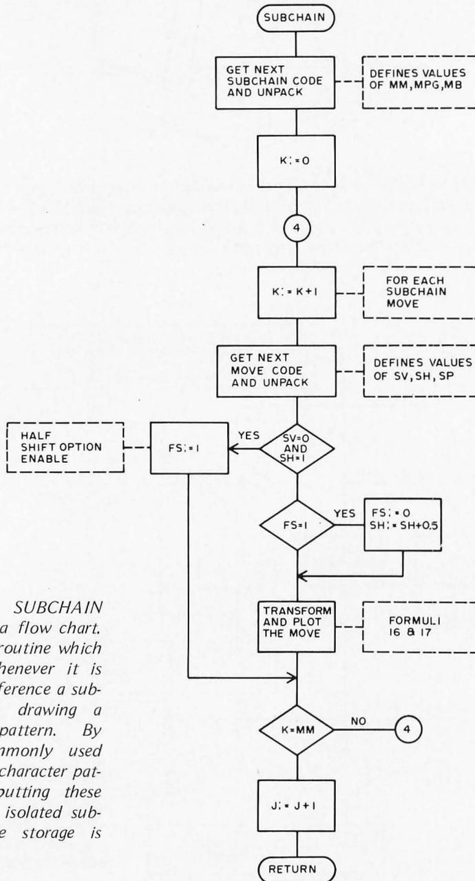
Figure 7: SUBCHAIN specified as a flow chart. This is a subroutine which is called whenever it is desired to reference a sub-chain when drawing a character pattern. By picking commonly used segments of character patterns and putting these segments in isolated sub-chains, table storage is conserved.
