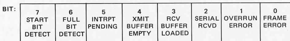
Figure 3: Status Word Format. The data read into the processor when TMS-5501 address location XXX3 is referenced is in this format.
