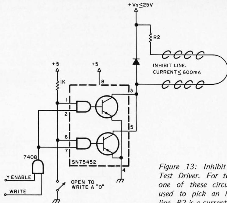
Figure 13: Inhibit Line Test Driver. For testing, one of these circuits is used to pick an inhibit line. R2 is a current limiting resistor set as described in the text of the article.
