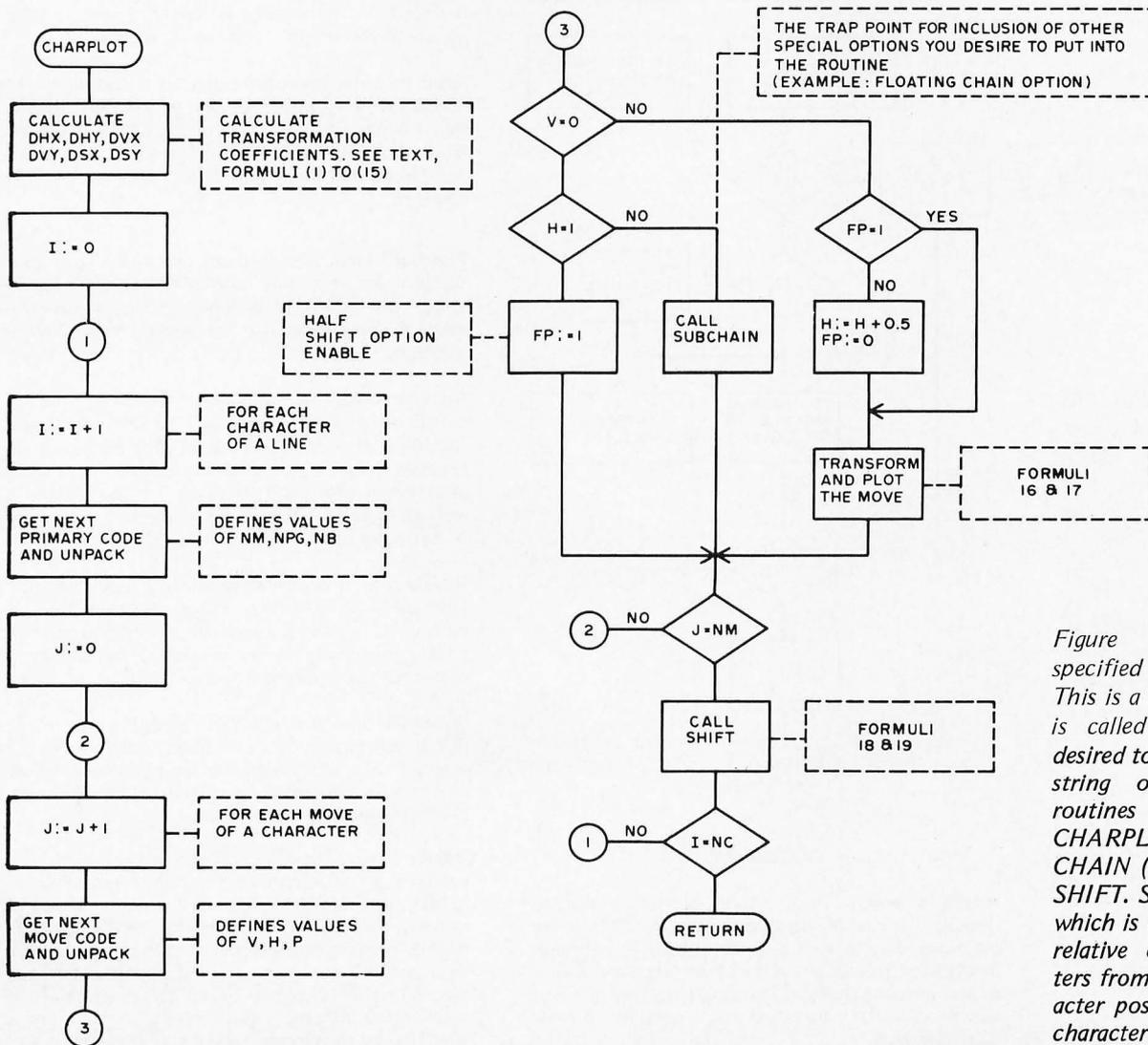
Figure 6: CHARPLOT specified as a flow chart. This is a subroutine which is called whenever it is desired to draw a character string of output. Subroutines referenced by CHARPLOT are: SUBCHAIN (see figure 7) and SHIFT. SHIFT is a routine which is used to move the relative origin of characters from the present character position to the next character position.
