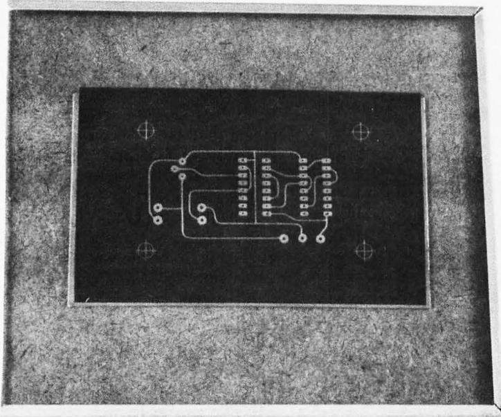
*Photo 2: Printing the Circuit. Once a negative of the artwork has been created, the next step is to print the circuit. The negative is placed over a sensitized PC board and held firmly in place by a glass cover plate in the printing frame. The glass guarantees smooth and even contact for accurate transfer of the image. The board is then exposed to a photoflood lamp for one to three minutes.*
