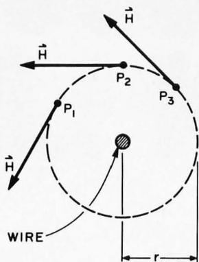
Figure 1: For a wire carrying current  $i$  directed out of the page, the magnetic field  $\mathbf{H}$  is proportional to  $i/r$ . The direction of  $\mathbf{H}$  is tangential to the circle of radius  $r$ , as shown for points  $P_1$ ,  $P_2$  and  $P_3$ .
