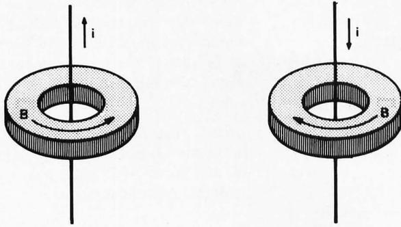
Figure 2: The direction of magnetic induction  $\mathbf{B}$  in the core results from alignment of core structures with the magnetic field due to current  $i$ .
