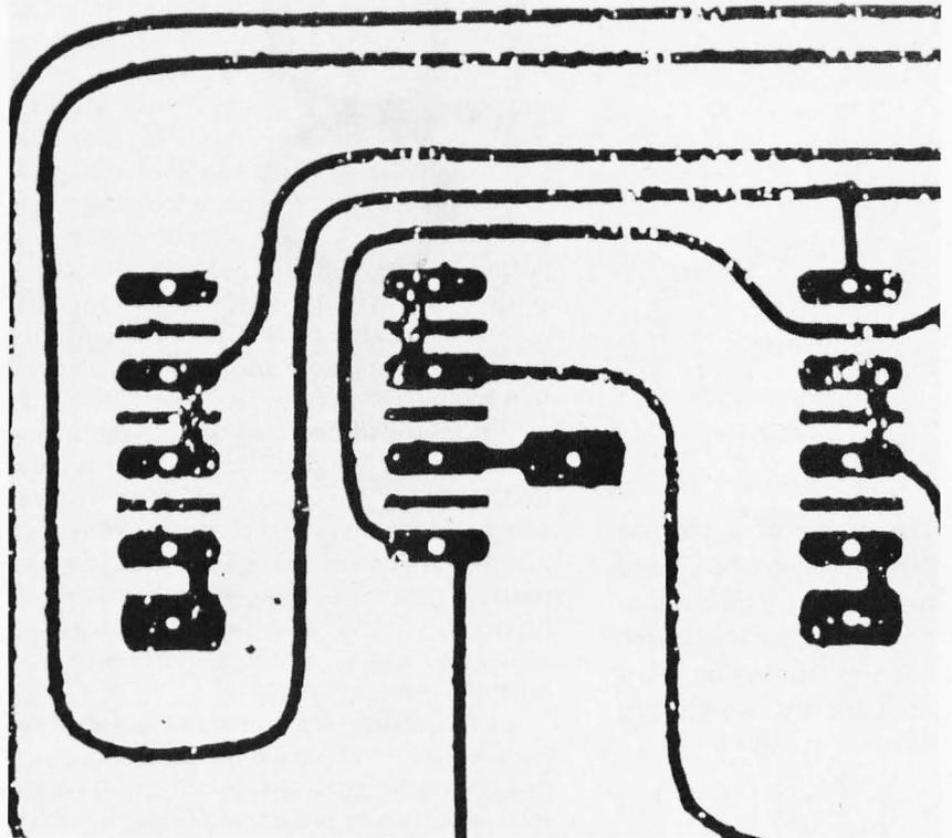
*Photo 9: When various imperfections enter the picture, the result is not so clean. Here is a high contrast picture of an imperfect result. The resist layer has separated from the copper during the etch process at several points, resulting in holes in the copper and, in several instances, complete breaks in circuit runs.*
